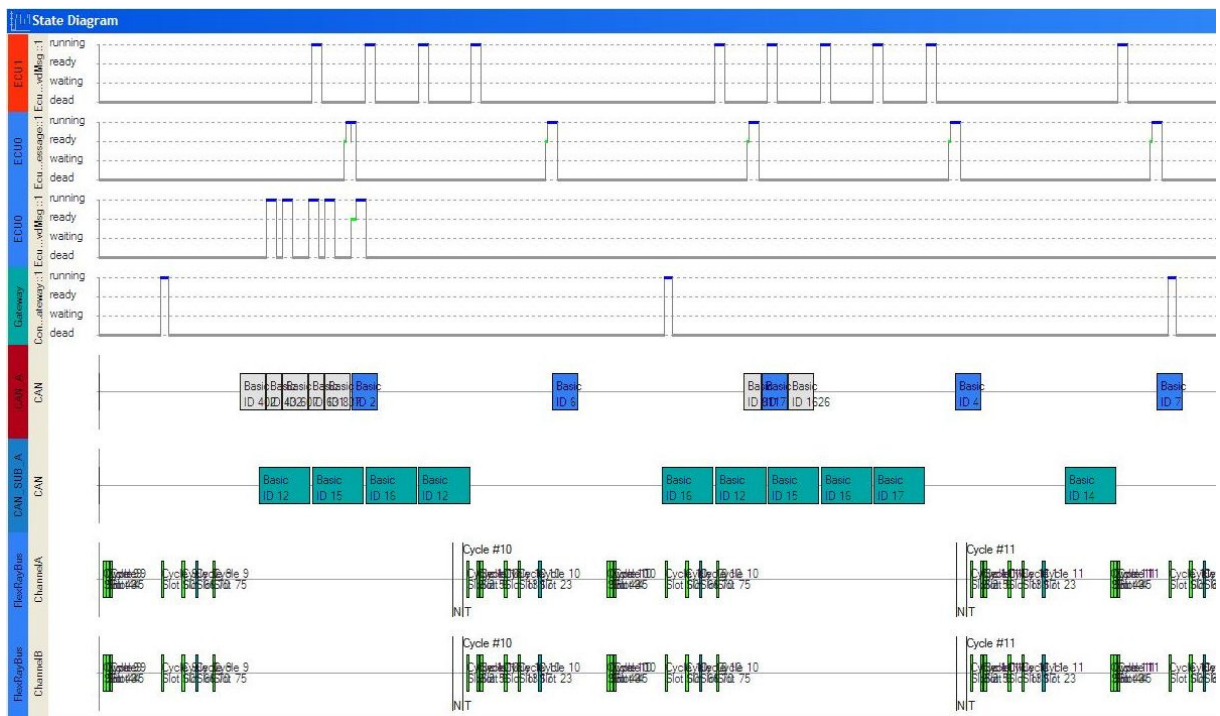
Figure 4: Task states of multiple ECUs combined with CAN and FlexRay communication
